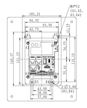
The following figures illustrate the positioning of the holes for mounting and the method of mounting.
