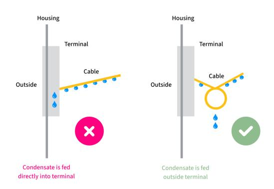
The occurrence of condensation moisture can be limited by avoiding rapid temperature and humidity condition changes or by avoiding direct flow of cold air onto the device.
